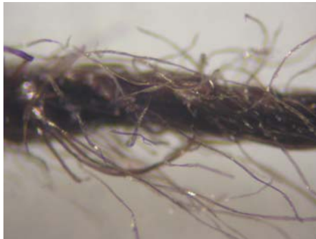
Figure 13: Lower thread (200x3dtex corespun cotton/polyester: coded as thread 2) used in fabric C
