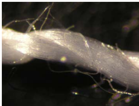
Figure 10: Upper thread (290x2dtex spun polyester: coded as thread 1) used in fabric A
