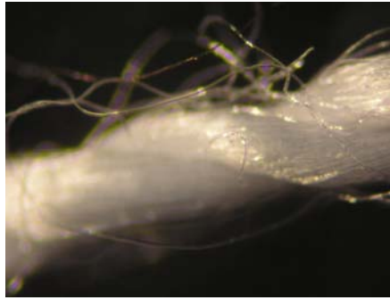
Figure 11: Lower thread (290x2dtex spun polyester: coded as thread 1) used in fabric A
