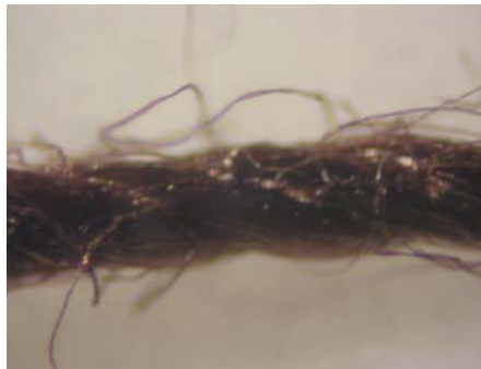
Figure 12: Upper thread (200x3dtex corespun cotton/polyester: coded as thread 2) used in fabric C
