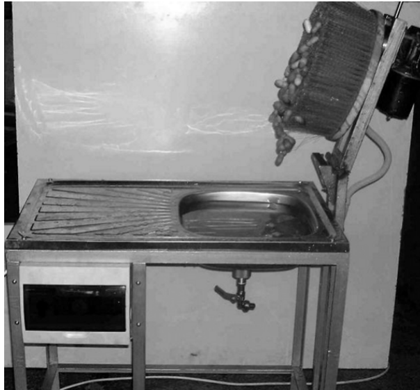
Figure 5 Installation for the friction of the silk cocoons
