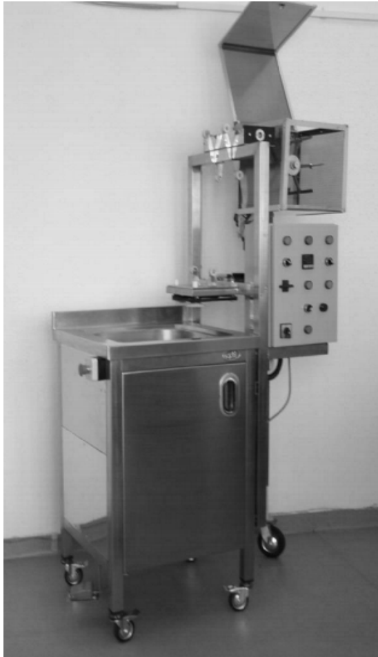
Figure 6 Installation for the spinning of the natural silk cocoons
