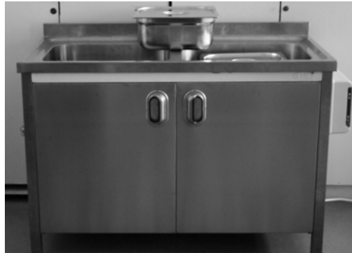
Figure 1: Installation for the boiling and storage of the boiled silk cocoons
